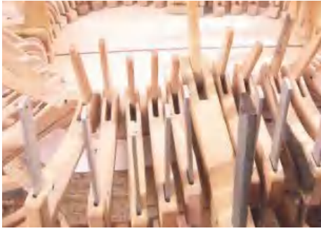
STEP 35. Clamping the back in place
